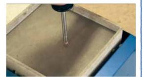
Press in the insert nut into the resin.
