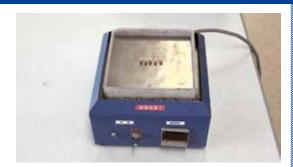
When insert nuts become relatively red brown, it is the time to start the inserting operation.
