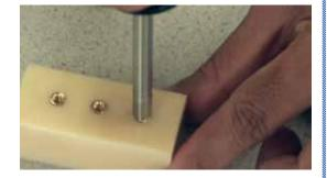
Press in till the set position, and pull out the insert driver slowly.
